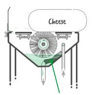
**Set washing water level:** enables washing where running water is not available – you simply fill up the water container (optional natural purifier (baking soda), water can be changed as necessary etc.).
