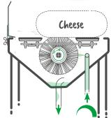
Set fresh water supply: washing with only fresh water provides the highest quality of washing. You can set the speed of rinsing the brush by opening and closing the valve.
