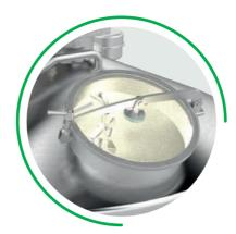
Glass Manhole Enables safe visual process monitoring.
