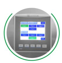
Automatic pressing regulation Automatic switching between 3 pre-set pressures and duration times. You can save 4 different programs with 3 steps.
