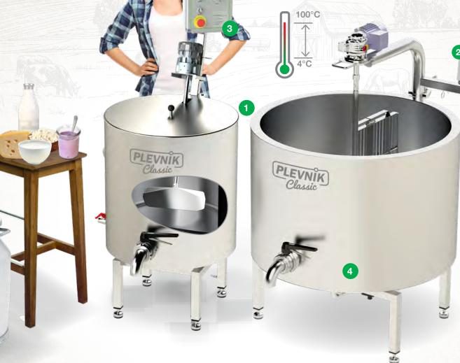
The 50I and 125I versions of the Classic model feature a double-coat insulated vessel with a cover and is made of AISI 304 stainless steel. Heating and cooling works through the bottom and the coat of the vessel. The kettle is heated in a water bath and cooled with water from the water supply network or a reservoir. Thermal treatment is possible up to 92°C. The temperature can be regulated using the thermostat on the electrical cabinet.
