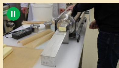
The butter is pressed into desired shape by turning the handle.
